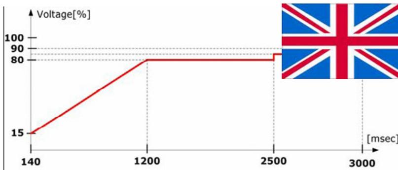
Figure 8. Fault-through-ride behaviour in United Kingdom [6]
