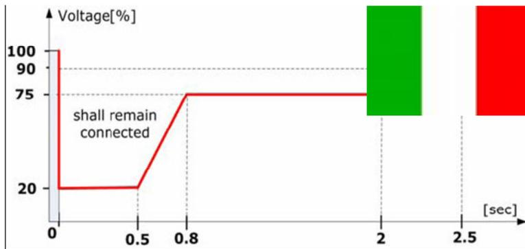
Figure 6. Fault-through-ride behaviour in Italy [6]
