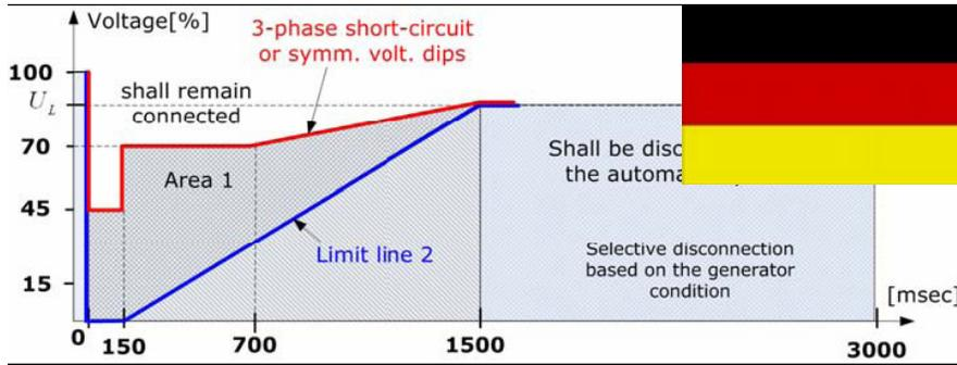
Figure 4. Fault-through-ride behaviour in Germany [6]
