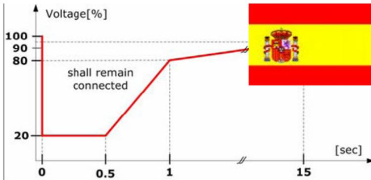
Figure 5. Fault-through-ride behaviour in Spain [6]
